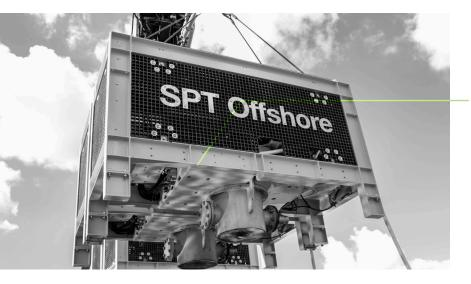
The SAPS-007 and SAPS-007S suction pump skids is part of our high-performance shallow-water suction pump systems. The SAPS-007 series are in particular suitable for the simultaneous installation of multiple suction piles like suction pile jacket foundations or suction pile cluster installations up to water depths of 150m. The individual control of the suction pressure and subsequent penetration in each pile makes accurate leveling possible. The main characteristics are:
