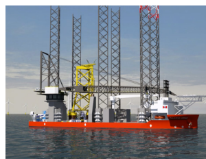
1. Transport WTG substructure on jackup vessel to field
