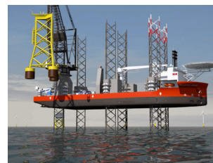
2. Position and lower to seabed
