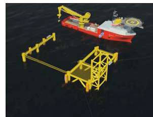
2. Ballast or lift to seabed and install suction pumps
