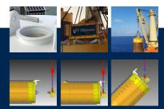
SPT OFFSHORE OWNS AND OPERATES REMOTELY CONTROLLED SUCTION PUMPS FOR WATER DEPTHS FROM 10M UP TO 3,000M. THESE PUMPS ARE PURPOSELY BUILT FOR THE INSTALLATION OF SINGLE PILES, SUCTION PILE CLUSTERS (SPCS), PLATFORM FOUNDATIONS OR SUBSEA STRUCTURE
