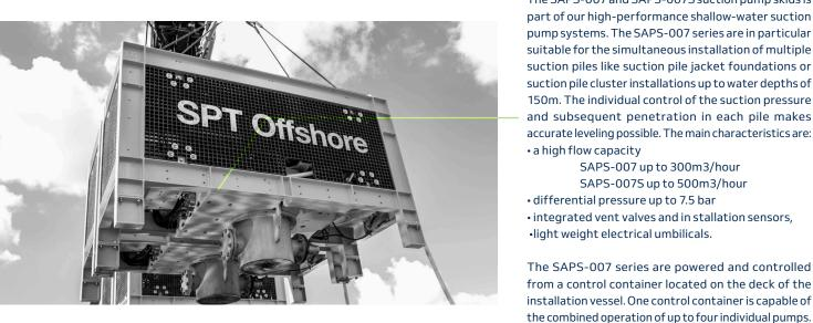
The SAPS-007 and SAPS-007S suction pump skids is part of our high-performance shallow-water suction pump systems. The SAPS-007 series are in particular suitable for the simultaneous installation of multiple suction piles like suction pile jacket foundations or suction pile cluster installations up to water depths of 150m. The individual control of the suction pressure and subsequent penetration in each pile makes accurate leveling possible. The main characteristics are: a high flow capacity
