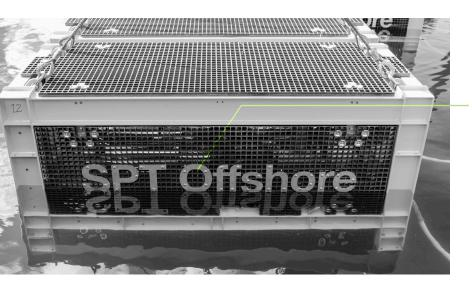
The SAPS-007L suction skid is part of our high-performance shallow-water suction systems. The SAPS-007 series are in particular suitable for the simultaneous installation of multiple suction piles like suction pile jacket foundations or suction pile cluster installations up to water depths of 150m. The individual control of the suction pressure and subsequent penetration in each pile makes accurate leveling possible. The main characteristics are:
