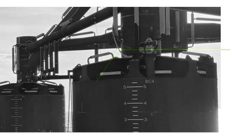
The SAPS-005 suction pump skids can be used for both shallow-water as deep-water suction pile installation. The SAPS-005 series are in particular suitable for either relatively small suction piles or suction pile clusters or for installations were installation speed is less critical. The individual control of the suction pressure and subsequent penetration in each pile makes accurate leveling possible.
