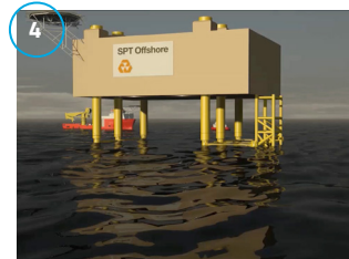
Install topsides by floatover or lift
