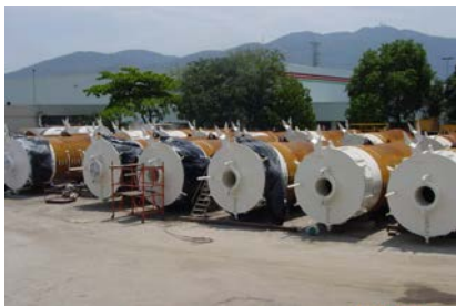
Fabrication of 22 suction piles in Brazil for the Chevron Frade project
