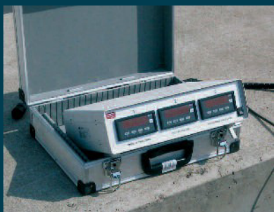
Monitoring unit pressure sensors
