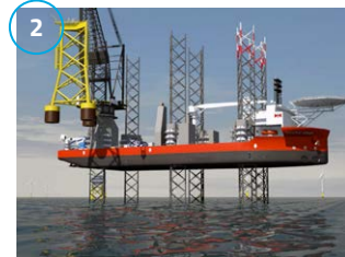
2 Position and lower to seabed
