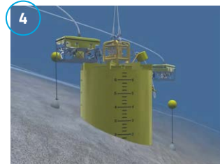
4 Lower to self weight penetration and close vent valve
