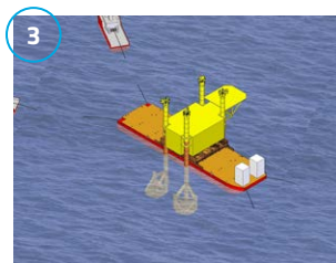
Lower legs and install suction piles
