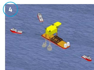
Lift deck and remove barge
